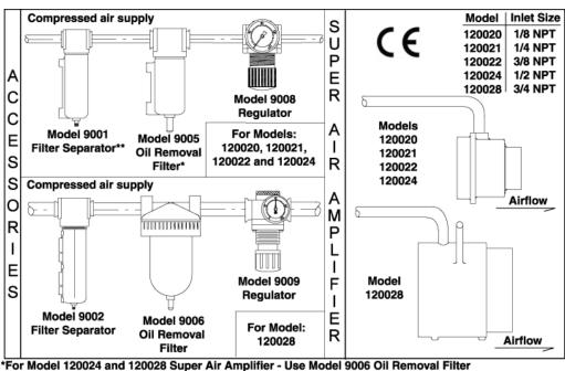
\*\*For Model 120024 and 120026 Super Air Ampliner - Use Model 9006 Oli Removal Filter \*\*For Model 120024 Super Air Amplifier - Use Model 9032 Filter Separator and Model 9033 Pressure Regulator
