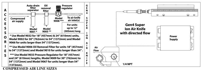
Compressed air lines should be sized to hold pressure drops to a minimum. Do not use restrictive fittings or undersized lines that can "starve" the Gen4 Super Ion Air Knife.
