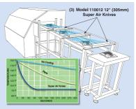
**Comment:** The laminar airflow of the Super Air Knives was the key to success in this application. Fan cooling could only provide random spikes of air at moderate velocities. **The uniform sheet of air from the Super Air Knife quietly swept the heat away within the first 2'** (**610mm**) of the conveyor. Low air consumption and the compact size of the Super Air Knife were an added bonus.
