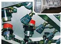
Model 120022 2" (51mm) Super Air Amplifiers and Model 1122 2" Flat Super Air Nozzles blow off transmissions after they are machined.
