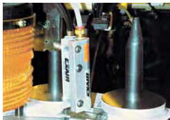
A Model 8103 3" (76mm) Gen4 Standard Ion Air Knife removes dust from computer hard disks prior to assembly.
