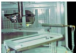
A Model 8212 12" (305mm) Gen4 Standard Ion Air Knife System cleans metal frames prior to powder coating.
