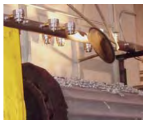
Metal parts are dried using a series of Model 6042 2" (51mm) Adjustable Air Amplifiers.
