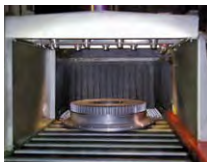
A series of Adjustable Air Amplifiers dry and cool a large machined casting as it exits a high temperature wash.
