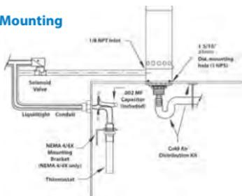
The Cabinet Cooler mounts to the enclosure through a drilled hole or electrical knockout. The NEMA 12 (IP54) Cabinet Coolers may be mounted on the top or side of the panel. NEMA 4 and 4X (IP66) Cabinet Coolers must be mounted on the top of the panel or on the side of the panel using one of our Side Mount Kits (See page 211).
