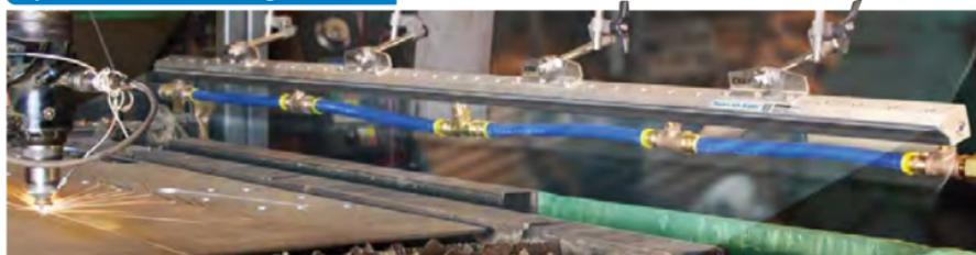
EXAIR offers Super Air Knives in lengths from 24" (610mm) through 108" (2743mm) with Plumbing Kits that are shipped fully assembled. All components have been properly sized to obtain the best performance from the Super Air Knife.
