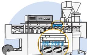
A Model 110006 6” (152mm) Super Air Knife opens pouches on a form-fill-seal-bagger.
