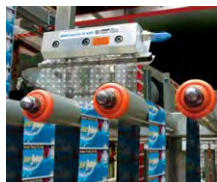
The Gen4 Super Ion Air Knife eliminates the static charge on labels being applied to PET soft drink bottles.
