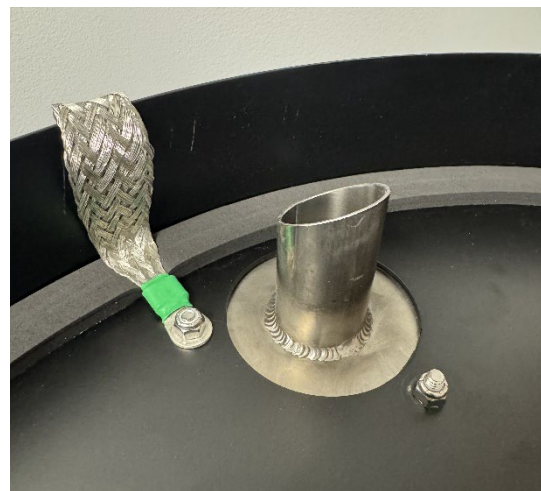
Figure 4: Bottom View of Ground Strap Installation
